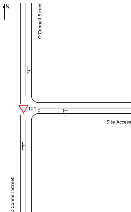
Figure 6.4 – Indicative O'Connell Street Access Layout
